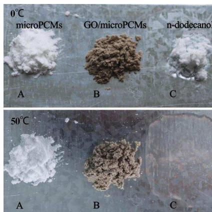
**Fig. 5** Digital photos of (A) microPCMs without GO, (B) GO/microPCMs, (C) n-dodecanol at different temperatures: 0 °C (upper) and 50 °C (lower).
