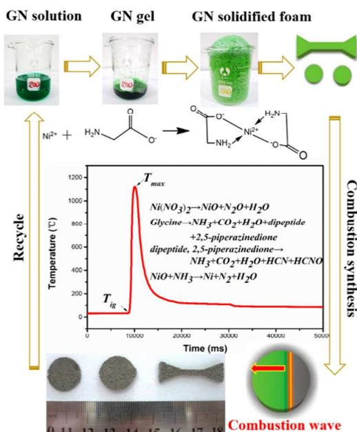
Figure 1 Schematic illustration of solid glycine-metal-nitrate self-propagation combustion route to continuous porous nickel monoliths.
