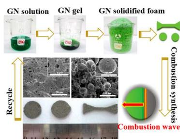
A novel solid metal-organic self-propagation combustion route to hierarchically porous metal monoliths with tunable chemistry, topography and microstructures.
