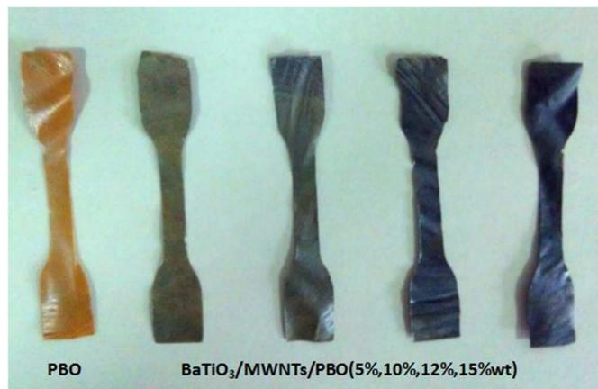
**Figure 6.** Tensile testing samples of the PBO and BaTiO<sub>3</sub>/MWNTs/PBO films with specified BaTiO<sub>3</sub>/MWNTs-loading (wt%).
