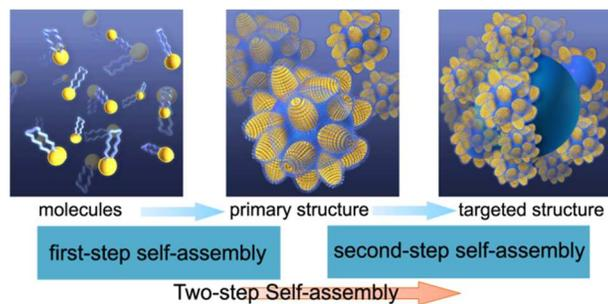
In this highlight, we proposed the concept of two-step self-assembly approach for the synthesis of hierarchically-ordered multifunctional nanostructures.
