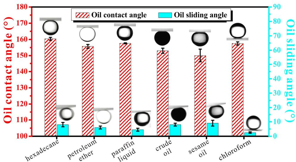
**Figure 7.** Underwater superoleophobicity and ultralow oil-adhesion of the femtosecond laser ablated silica glass surface ( $AD = 4 \mu\text{m}$ ) for various oils in terms of their oil contact angles and oil sliding angles, respectively.
