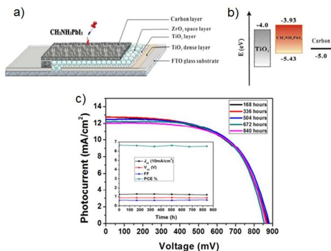
**Figure 4** – (a) The structure of the first carbon counter electrode based PSC.<sup>64</sup> (b) Energy level of TiO<sub>2</sub>, CH<sub>3</sub>NH<sub>3</sub>PbI<sub>3</sub> and carbon.<sup>64</sup> (c) Current density–voltage curves of carbon cathode based PSCs over 840 hours. Inset: the effect of time on each value ( $J_{sc}$ ,  $V_{oc}$ , FF and PCE) of solar cell. Reprinted with permission from ref. 64 © 2013, Nature Publishing Group.
