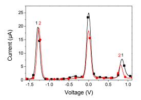
Fig. 1 Square wave voltammogram of 1 (black line) and 2 (red line). The potential is referenced to ferrocene/ferrocenium redox couple = 0.0 V.
