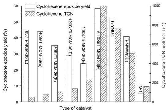
**Figure 13.** Epoxide yield and turnover number for the epoxidation of cyclohexene over xSi/Ti-MCM-36(E), Ti-YNU-1, Ti-MWW and TS-1. Reaction conditions: 0.05 g of catalyst, 10 mmol of alkene, 5 mmol of TBHP (60 wt %), 3 mL of decane solvent, 353 K, 2 h.
