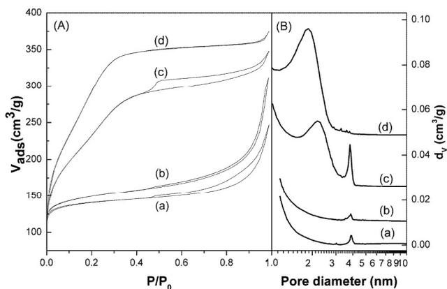
**Figure 4.** (A)  $N_2$  adsorption/desorption isotherms and (B) BJH pore size distribution of (a) ERB-1, (b) MCM-22, (c) 40Si/Ti-MCM-36(M), and (d) 40Si/Ti-MCM-36(E).
