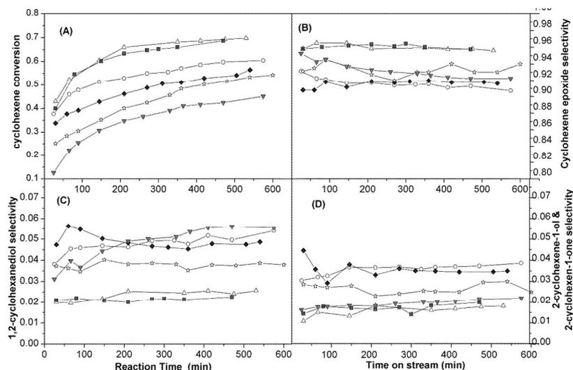
**Figure 12.** (A) Cyclohexene conversion, (B) cyclohexene epoxide selectivity, (C) 1,2-cyclohexanediol selectivity and (D) 2-cyclohexene-1-ol selectivity vs TOS for ( $\Delta$ ) A-Si/Ti-MCM-36(E), ( $\blacksquare$ ) Ti-YNU-1, ( $\circ$ ) 40Si/Ti-MCM-36(E), ( $\blacklozenge$ ) 80Si/Ti-MCM-36(E), ( $\star$ ) 120Si/Ti-MCM-36(E) and ( $\blacktriangledown$ ) 140Si/Ti-MCM-36(E).
