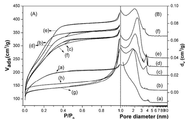
**Figure 8.** (A) N<sub>2</sub> adsorption/desorption isotherms (B) BJH pore size distribution of (a) 0Si/Ti-MCM-36(E), (b) 40Si/Ti-MCM-36(E), (c) 80Si/Ti-MCM-36(E), (d) 120Si/Ti-MCM-36(E), (e) 140Si/Ti-MCM-36(E), (f) A-Si/Ti-MCM-36(E), (g) Ti-MWW and (h) Ti-YNU-1.
