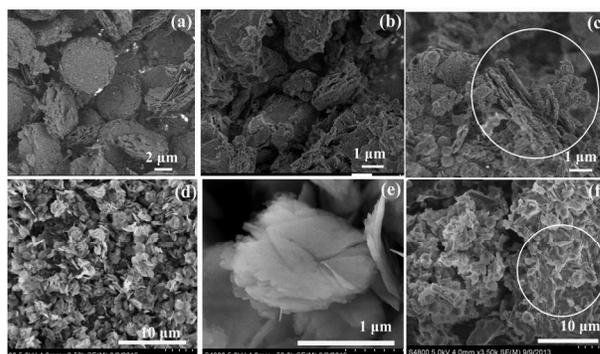
**Figure 1.** The scanning electron micrographs of (a) calcined ERB-1, (b) and (c) 40Si/Ti-MCM-36(E) from JEOL JSM-7600F, (d) and (e) calcined MCM-22; (f) 40Si/Ti-MCM-36(M) from Hitachi S-4800 Field Emission Scanning Electron Microscope.
