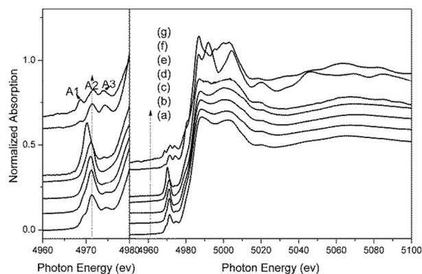
**Figure 9.** Ti *K*-edge XANES of (a) 0Si/Ti-MCM-36(E), (b) 40Si/Ti-MCM-36(E), (c) 140Si/Ti-MCM-36(E), (d) A-Si/Ti-MCM-36(E), (e) Ti-YNU-1, (f) rutile and (g) anatase TiO<sub>2</sub>.
