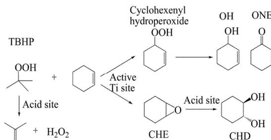
**Scheme 1.** Reaction scheme of epoxidation of cyclohexene and possible by-products.
