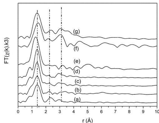
**Figure 10.** Fourier transform *k*<sup>3</sup>-weighted Ti EXAFS spectra in *R*-spacing of (a) 0Si/Ti-MCM-36(E), (b) 40Si/Ti-MCM-36(E), (c) 140Si/Ti-MCM-36(E), (d) A-Si/Ti-MCM-36(E), (e) Ti-YNU-1, (f) rutile and (g) anatase TiO<sub>2</sub>.
