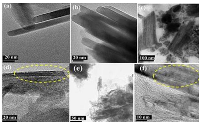
**Figure 2.** Transmission electron micrographs of (a) ERB-1(P), (b) MCM-22(P); (c), (d) 40Si/Ti-MCM-36(E), and (e), (f) 40Si/Ti-MCM-36(M). ((a), (b), (d), (f) from Philips/FEI Tecnai 20 G2 S-Twin, and (c), (e) from JEM-1200EX II Transmission Electron Microscope).
