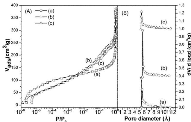
**Figure 5.** (A) log plots of Ar sorption isotherms and (B) Horvath-Kawazoe differential pore volume plots of (a) ERB-1, (b) 40Si/Ti-MCM-36(E) and (c) A-Si/Ti-MCM-36(E).
