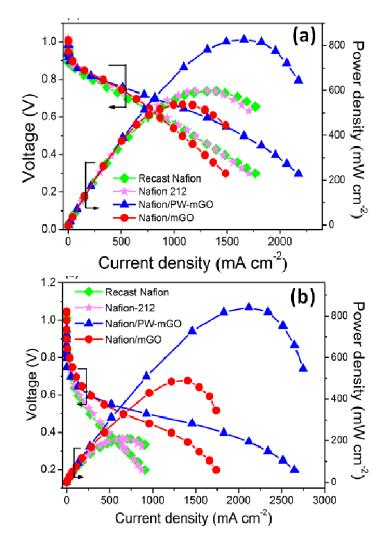
**Fig. 5**. Polarization and power density plots of (a) Nafion-212, recast Nafion, Nafion/mGO and Nafion/PW-mGO under 100%RH at 80 °C (b) operated under 20%RH at 80 °C. One weight percent filler content was used in composite membranes, catalyst loading in anode and cathode kept 0.5 mg/cm<sup>2</sup>.
