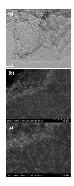
**Fig. 3** (a) TEM and (b, c) STEM-HAADF images of PW-mGO hybrid. Bright spots represent PW clusters are well dispered on graphene oxide surface.
