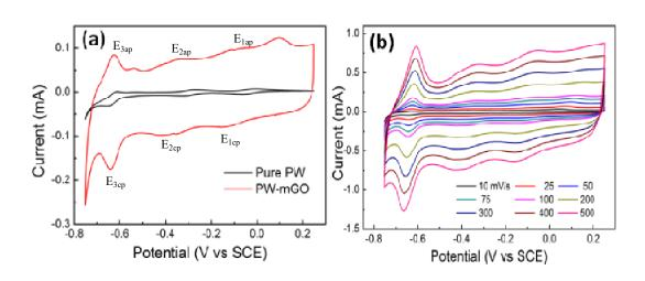
**Fig. 4** (a) The comparison of CV of pure PW and PW-mGO at 25 mVs<sup>-1</sup> scan rate in  $1 \text{ M H}_2\text{SO}_4$  electrolyte, (b) The effect scan rate of PW-mGO hybrid electrode.
