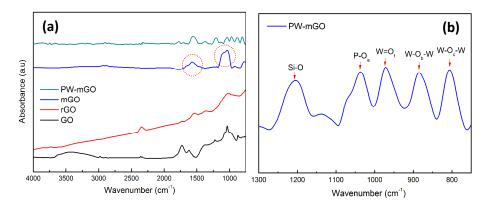
**Fig. 2** (a) FT-IR spectra of GO, rGO, mGO, PW-mGO, the red circle marked are –NH<sub>2</sub>, and Si-O-Si bond, (b) metal-oxide stretching peak information of PW-mGO.
