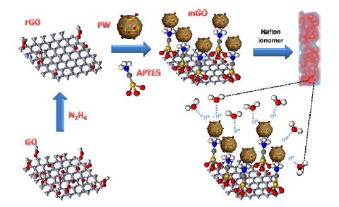
**Fig. 1** Schematic representation of fabrication of phosphotungstic acid modified reduced graphene oxide-Nafion composite membrane.
