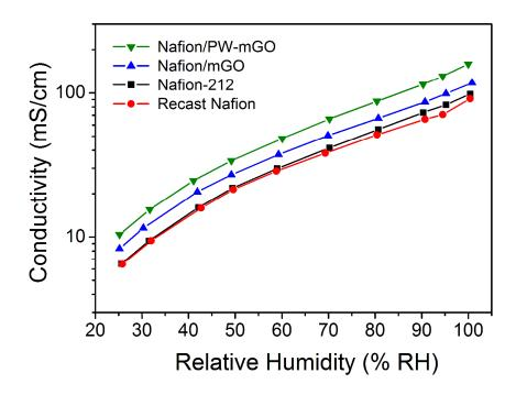
**Fig. 6.** Proton conductivity of Nafion-212, Nafion/mGO, and Nafion/PW-mGO composite membranes measured under different relative humidity at 80 °C
