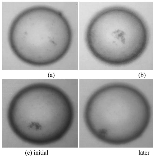
Figure 6. Distribution of polystyrene particles on silicone oil-I drop in castor oil. The mean particle diameter was 4  $\mu\text{m}$  and the drop diameter was around 400  $\mu\text{m}$ . Due to their small size, particles appear as dots in the images. The voltages and frequencies are (a) 0 V; (b) 4 kV at 4 Hz; (c) 4 kV at 40 Hz. The two photographs show particles migrating towards the equator.
