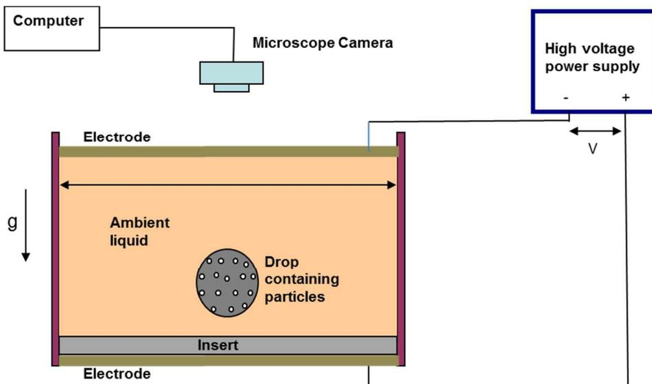
Figure 3. A schematic of the setup used in our experiments. The electrodes were mounted on the top and bottom of the device. The resulting electric field was in the vertical direction.
