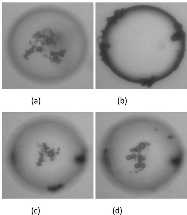
Figure 11. Distribution of hollow and solid glass particles on the surface of silicone oil-II drop immersed in castor oil. The mean diameter of the hollow and solid glass particles was  $18 \mu\text{m}$  and  $2 \mu\text{m}$ , respectively, and the drop diameter was  $405 \mu\text{m}$ . The voltages and frequencies are (a) 0 V; (b) 2 kV at 0.2 Hz; (c) 4 kV at 10 Hz (d) 4 kV at 20 Hz.
