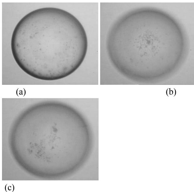
Figure 5. Distribution of soda lime glass particles on silicone oil-I drop in castor oil. The mean particle diameter was about 2  $\mu\text{m}$  and the drop diameter was 400  $\mu\text{m}$ . Particles appear as small dots in the photographs due to their small size. Particles collected at the poles as both the DEP
