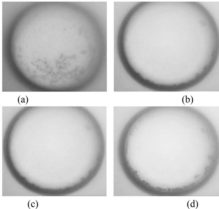
Figure 8. Distribution of solid glass particles on silicone oil-II drop in castor oil. The mean particle diameter was 4  $\mu\text{m}$  and the drop diameter was around 430  $\mu\text{m}$ . Due to their small size, particles appear as dots in the images. In (b)-(d) they are concentrated near the equator. The voltages and frequencies are (a) 0 kV; (b) 2 kV at 0.2 Hz; (c) 4 kV at 1 Hz; (d) 4 kV at 120 Hz. The photographs show that in (b)-(d) particles collected near the equator.
