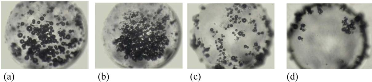
Figure 10. Distribution of hollow and solid glass particles on the surface of a silicone oil-I drop immersed in castor oil. The mean diameter of the hollow and solid glass particles was 18  $\mu\text{m}$  and 2  $\mu\text{m}$ , respectively, and the drop diameter was 430  $\mu\text{m}$ . The voltages and frequencies are (a) 0 V; (b) 2 kV at 0.4 Hz; (c) 3 kV at 6 Hz (d) 3 kV at 20 Hz.
