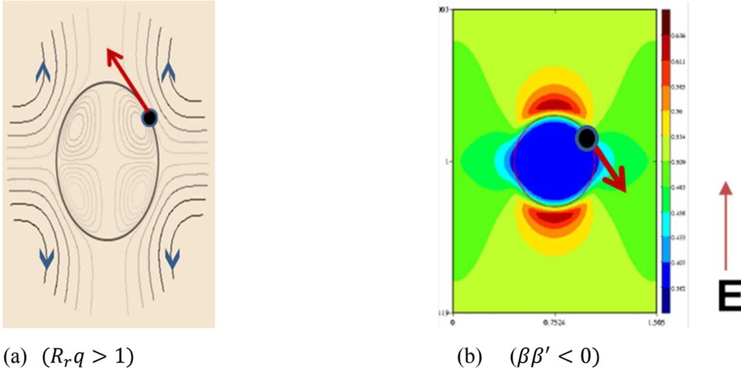
Figure 1. Streamlines of EHD flow in a leaky dielectric fluid which determine the direction of EHD force and isovalues of electric field intensity which determine the direction of DEP force: (a) streamlines of EHD flow for  $R_r q > 1$ , (b) isovalues of the electric field intensity around a drop subjected to a uniform electric field generated by the electrodes placed at the top and
