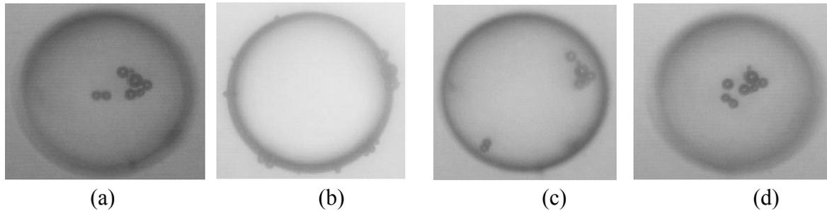
Figure 7. Distribution of hollow glass particles on silicone oil-II drop in castor oil. The mean particle diameter was 18  $\mu\text{m}$  and the drop diameter was around 400  $\mu\text{m}$ . The voltages and frequencies were (a) 0 V; (b) 3 kV at 0.2 Hz; (c) 3 kV at 16 Hz; (d) 8 kV at 20 Hz.
