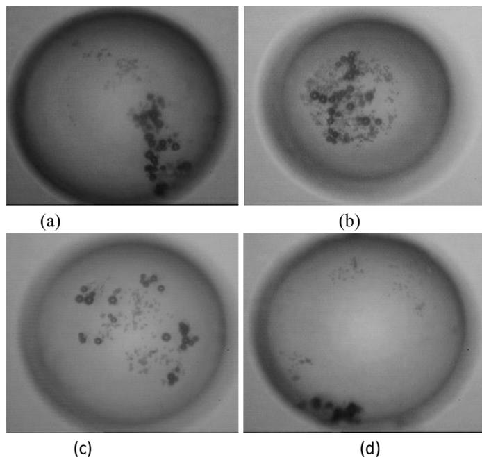
Figure 9. Distribution of a mixture of hollow glass and polystyrene particles on a silicone-I oil drop immersed in castor oil. The mean diameter of the glass and polystyrene particles was 18  $\mu\text{m}$  and 4  $\mu\text{m}$ , respectively, and the drop diameter was 410  $\mu\text{m}$ . The voltages and frequencies were (a) 0 V; (b) 2.5 kV at 0.1 Hz; (c) 3 kV at 6 Hz (d) 3 kV at 20 Hz.
