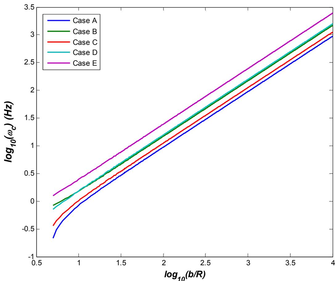
Figure 2. The critical frequency at which the EHD and DEP forces are equal as a function of  $\frac{b}{R}$  for cases A-E described in Table 3.
