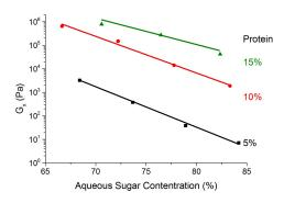
**Fig. 9** The dependence of the cross-over modulus,  $G_{\times}$  on the (sugar:water) ratio at the standard oil fraction for three different protein concentrations. Lines are exponential fits.
