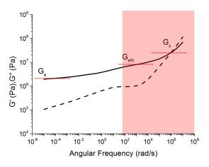
**Fig. 6** Ferry's 'type VII' master curves for a 'very lightly cross-linked amorphous polymer', here a vulcanised styrene-butadiene random copolymer. The shaded part corresponds to the caramel master curves in Fig.5. Solid lines: G', dashed lines: G''.
