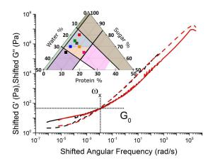
**Fig. 5** Overlay of two master curves obtained using tCS on the two sequence of samples shown as points in the inset, with spectra shifted related to the reference sample common to the two sets. Solid lines: G', dashed lines: G''. Compositions are Red: superposition of 5%P caramels; Black: superposition of 20%W caramels.
