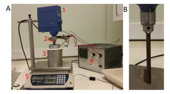
**Fig. 1** A. Our caramel apparatus. Contents are stirred by an IKA mixer (1) rotating a blade (2). An aluminium cylinder is heated by a jacket with embedded resistors (3). The temperature is controlled via a PID controller (4), The whole vessel is on a balance (5) to monitor water boil off. B. Detailed view of the mixing blade with gap for thermocouple.
