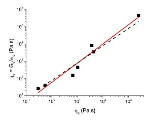
**Fig. 8** The cross-over viscosity,  $\eta_\times = G_\times \omega_\times^{-1}$  of a number of caramels plotted against the measured viscosity of the background sugar solution in each sample. Red line: best fit to  $\eta_\times = \eta_0 \eta_s^\beta$  with  $\eta_0 = 59$  (Pa.s) $^{-0.1}$  and  $\beta = 1.1 \pm 0.1$ . The black dashed line has unit slope.
