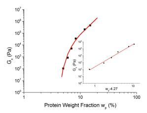
**Fig. 10** The dependence of the cross-over modulus,  $G_{\times}$  on protein concentration, w, at the standard oil fraction and a constant sugar:water ratio of 2.9. The error bars for these data points are the size of the points or lower. The red curve is a fit to  $G_{\times} \sim \mathfrak{G}(w-w_c)^f$ , Eq. 6, with  $\mathfrak{G}=318$  Pa,  $w_c=4.27\%$  and f=3.17. The inset shows the same data and fitting in a plot against  $\log(w_p-4.27\%)$ .
