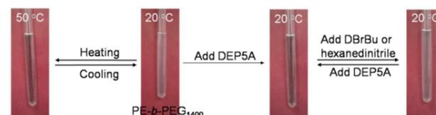
**Fig. 2** PE-*b*-PEG<sub>1400</sub> in  $\text{CDCl}_3$  (10.0 mg/mL) and its tuning processes by heating and adding DEP5A or competitive guest molecule of DBrBu or hexanedinitrile.
