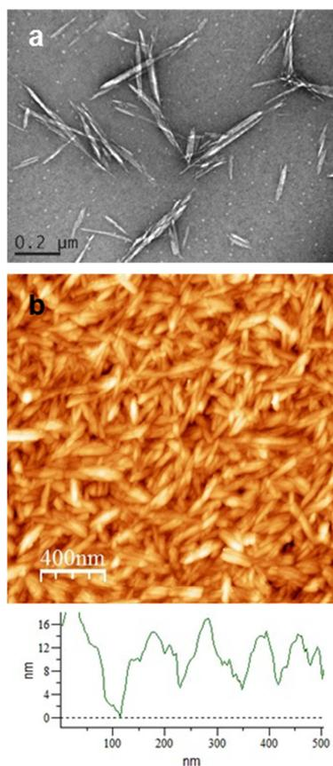
Fig. 2 TEM micrograph of negatively stained cellulose nanocrystals (a), and representative  $2 \times 2 \mu\text{m}^2$  AFM topographical image of the spin-coated one-layer film of CNC at  $3 \text{ g L}^{-1}$  (b) onto a silicon wafer.
