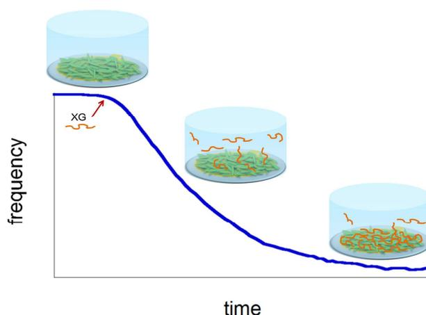
Fig. 1 Schematic illustration of XG adsorption onto spin-coated CNC surfaces monitored by quartz crystal microbalance.
