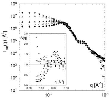
**Figure 4**: Double logarithmic plots of the normalized scattered intensity of PDMA/silica hydrogels (SPx\_PW0.14\_R0.1) prepared in solvent p (silica scattering) with different amount of silica: SP0.5 ( $\nabla$ ), SP1 ( $\triangle$ ), SP2 ( $\triangle$ ), SP3.5 (O) and SP4.8 ( $\bigcirc$ ). **Inset:** Experimental structure factor obtained by dividing the reduced scattering intensity of hybrid formulations by the reduced scattering intensity of dilute silica suspension ( $\phi_f = 0.0044$ ).
