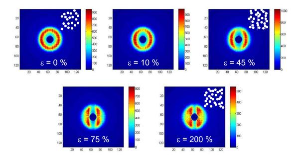
**Figure 6**: 2D-SANS images of a step-by-step loading of SP5\_PW0.14\_R0.1 hybrid hydrogel. The white dots in the upper right corner schematically picture the average distance between silica particles in hybrid hydrogels for un-stretched ( $\varepsilon = 0\%$ ) and stretched materials, before ( $\varepsilon = 45\%$ ) and during ( $\varepsilon > 75\%$ ) shear reorganization. The dotted lines shown at  $\varepsilon = 45\%$  highlight the alignment of particles under transverse compression.
