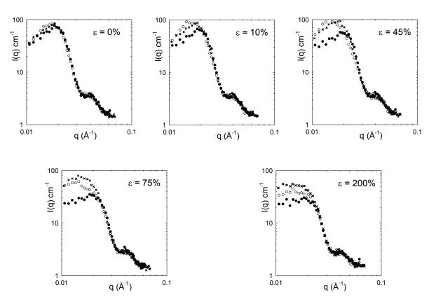
**Figure 7**: Double logarithmic plot of the scattering intensity of SP5\_PW0.14\_R0.1 hydrogel studied at different strains: from 0% to 200%. The data were obtained from 2D-SANS images according to different sector-averaging patterns of  $10^{\circ}$ width:  $0^{\circ}$  ( $\bigcirc$ ),  $45^{\circ}$  (X) and  $40^{\circ}$  ( $\bigcirc$ ).
