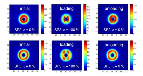
**Figure 9**: 2D-SANS patterns of SP2\_PW0.14\_R0.1 (up) and SP5\_PW0.14\_R0.1 (down) hybrid hydrogels before loading ( $\varepsilon = 0\%$ ; left), under loading (middle;  $\varepsilon = 100\%$ ) and after unloading (right;  $\varepsilon = 0\%$ ).
