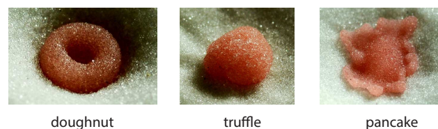
Fig. 1 Various crater morphologies observed in the experiments are categorized as: doughnut, truffle, and pancake.
