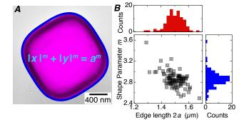
Fig. 1 Colloidal Superballs (A) Sample TEM image showing a hollow silica superball. The blue line shows a fit of the edge contour to  $|x|^m + |y|^m = a^m$  to extract the shape parameter m and edge length 2a. (B) Scatter plot of the shape parameter and edge length extracted from 96 TEM images from a single batch of cubes. Bar plots above and to the right show histograms of the same data.
