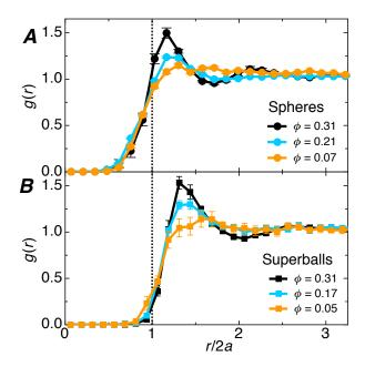
**Fig. 4** Microstructure of superball and hard sphere suspensions. Pair distribution function g(r) for suspensions of (A) superballs and (B) PMMA spheres at various volume fractions  $\phi$ . The separation distance r is scaled by the average diameter  $2a = 1.45 \mu m$  for the PMMA spheres and by the average edge length  $2a = 1.50 \mu m$  for the superballs. Error bars reflect the standard deviation reflect the standard deviation from multiple measurements with the same sample.
