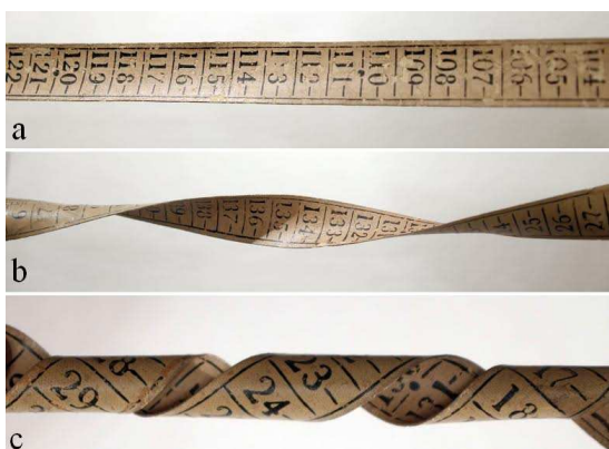
Fig. 7 Analogy of ribbon, helicoidal and tubular state for a measuring tape. Grabbing the tape (a) by the ends and twisting it slightly, we put it into a helicoidal conformation (b). A somewhat larger twist induces a transition into the helical state (c). The difference between (b) and (c) lies in that in (b) the center line of the ribbon is straight and coincides with its symmetry axis, whereas in (c) the center line is a helix itself.
