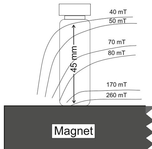
**Fig. 1** Sketch of the permanent magnet and the lines (surfaces) of constant field strength, as indicated, which have been previously mapped out using a Hall probe. The sample was placed always at the same marked position near the edge of the magnet. The resulting gradient of the magnetic field is roughly 5 T/m.
