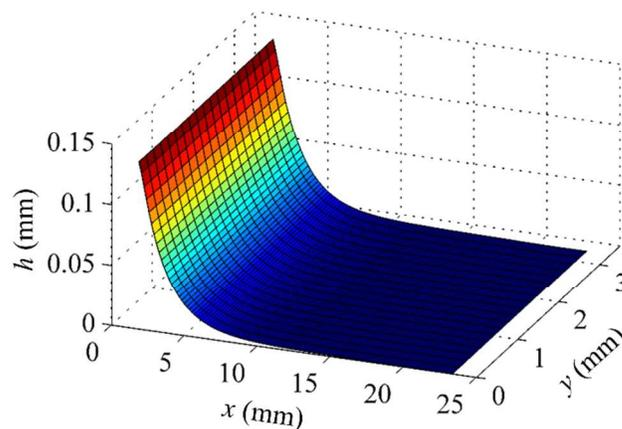
Fig. 6: Three-dimensional (3D) profile of dodecane meniscus on an inclined plate.
