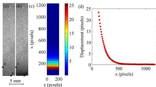
Fig. 5 (a) image of the background pattern with plane dodecane surface, (b) image of the background pattern with meniscus, (c) computed displacement field, and (d) displacement magnitude  $\mathbf{M}'\mathbf{M}''$  as a function of distance from the inclined plate.
