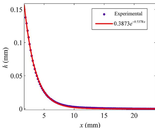
Fig. 7: Experimentally measured meniscus profile and fitted curve.
