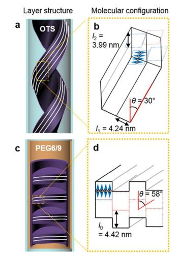
**Figure 4.** Schematic sketch of  $HNFs_{(mod)}$  and bamboo-like B4 structures from W618 in OTS- and PEG 6/9-treated AAO nanochannels. a, b, On the OTS-coated nanochannel surface, discrete rectangular columnar unit cells slid to form pseudo-layers<sup>20</sup> and finally formed  $HNF_{(mod)}$ . c, d, On the PEG 6/9-coated surface, discrete rectangular columnar unit cells were held in the molecular-philic nanochannel wall and crystallized, maintaining their lattice upon cooling.
