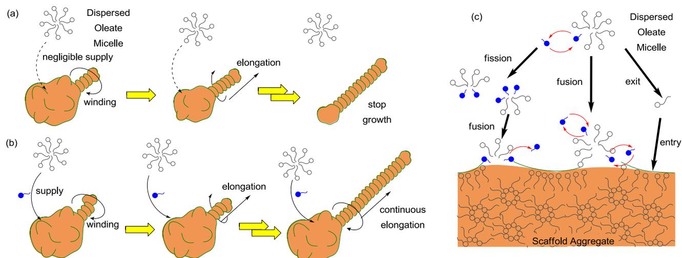
**Figure 9.** Schematic illustration for the elongation of helical assemblies of oleates (a) without and (b) with medium-chain aliphatic acids (indicated by blue color). (c) Three plausible mechanisms, fission-fusion, fusion, and exit-entry, for mediator-assisted molecular supply to the terminal scaffold.
