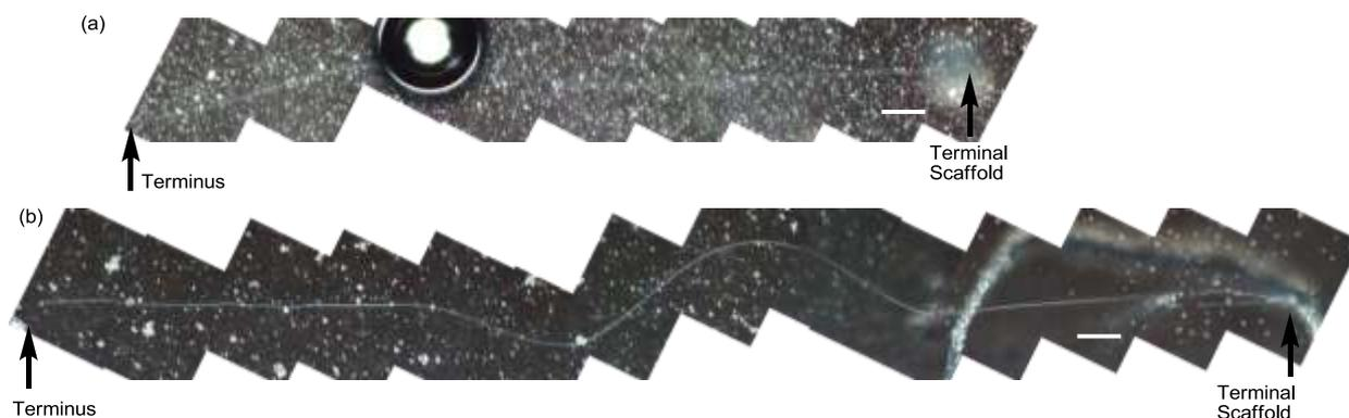
**Figure 3.** Helical assemblies of oleates formed in the presence of fatty acids. (a) ~2-millimeter-long assembly in the presence of sodium pelargonate ( $C_9Na$ , 1% (w/w)). (b) ~3-millimeter-long assembly in the presence of sodium caprate ( $C_{10}Na$ , 1% (w/w)). Bars indicate 0.1 mm.
