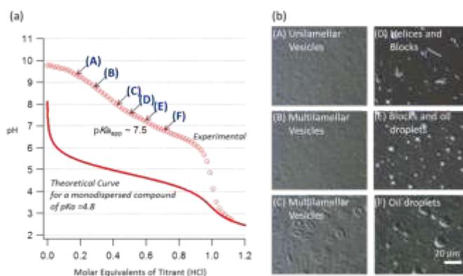
**Figure 4.** (a) Titration curve of 6.6 mM **ONa** in 0.1 M NaCl(aq), with 0.5 M HCl(aq) as the titrant (circles). The line shows the curve calculated by the Henderson–Hasselbalch equation for the sodium salt of a water-soluble acid ( $pK_a = 4.8$ ), considering the experimental conditions, including ionic strength. (b) Micrographs of assemblies collected at the pH values in (a).
