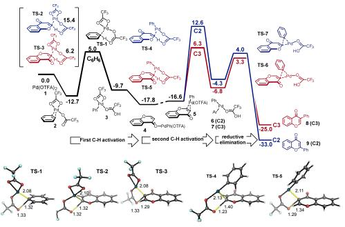
Figure 2. Coupling of chromone and benzene via sequential C-H activation. Palladation of benzene (40-fold excess) with Pd(OTFA)<sub>2</sub> is marginally faster than for the C3-position of chromone; Palladation of chromone by PhPd(OTFA) and subsequent reductive elimination: the C3-regioselectivity afforded by this mechanism is inconsistent with experiment. Structures are colored as follows: Pd(dark blue), F(light blue), O(red), C(grey), H(white).
