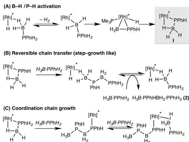
**Scheme 12.** Suggested mechanisms for dehydropolymerization. [Rh] = Rh(PR<sub>3</sub>)Cp\* (PR<sub>3</sub> = PMe<sub>3</sub> or PPhH<sub>2</sub>).
