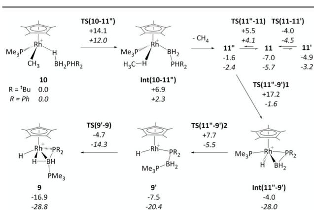
**Figure 5:** Computed free energy reaction profile (kcal/mol, BP86-D3( $\text{CH}_2\text{Cl}_2$ ) level) for formation of **9** from **10** ( $\text{R} = \text{tBu}$ ) with equivalent data for  $\text{R} = \text{Ph}$  provided in italics. All free energies are quoted relative to **10** + free  $\text{H}_3\text{B-PHR}_2$  at 0.0 kcal/mol; see Figure 4 for details of species **11**, **11'** and **11''** when  $\text{R} = \text{tBu}$ .
