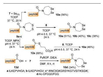
Scheme 4. Synthesis of SeEA peptides.\* The Cys residue is temporarily protected by a tert-butylsulfenyl (tBuS) group in 9c. It is removed during the exchange
