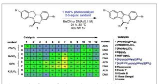
Figure 2. Identification of a photoredox-mediated dehydrogenation via high-throughput experimentation. Reactions performed on 2.5  $\mu$ mol scale using 465 nm LEDs. Numbers in table refer to assay yields based on HPLC analysis with an internal standard.
