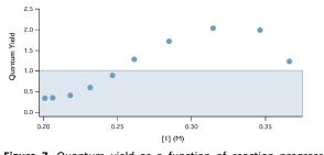
**Figure 7.** Quantum yield as a function of reaction progress using 0.1 mol% [Ir(dF-CF<sub>3</sub>-ppy)<sub>2</sub>(dtbpy)](PF<sub>6</sub>), 2 equiv. *t*BPB, 1 equiv. **1** in DMA.
