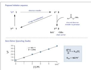
**Figure 11.** Proposed initiation sequence and Stern-Volmer quenching studies of **1** and [Ir(dF-CF<sub>3</sub>-ppy)<sub>2</sub>(dtbpy)](PF<sub>6</sub>).
