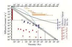
**Descriptive Statement:** Direct comparison of diffusion coefficients and viscosities of ternary component single aerosol particles levitated using optical tweezers.
