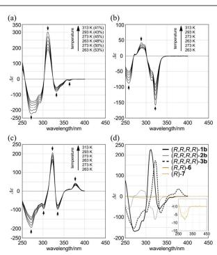
Figure 7. VT-CD spectra of (a) (R,R,R,R)-**1b**, (b) (R,R,R,R)-**2b**, and (c) (R,R,R,R)-**3b**, measured in CH<sub>2</sub>Cl<sub>2</sub> at 263-313 K. (d) CD spectra of (R,R,R,R)-**1b**, (R,R,R,R)-**2b**, single-stranded substructure (R,R)-6, and diphenylacetylene derivative (R)-7, measured in CH<sub>2</sub>Cl<sub>2</sub> at 293 K. In (a), helical excess (%) is noted in parenthesis.
