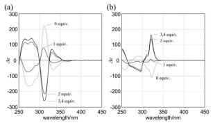
Figure 8. CD spectra of (a) (R,R,R,R)-**1b**  $(8.4\times10^{-5}\ \text{M})$  and (b) (R,R,R,R)-**2b**  $(1.0\times10^{-8}\ \text{M})$  in the presence of achiral ditopic guest **4** (solid lines) [0 (**1** only, dashed line), 1, 2, 3 and 4 equiv.]. All spectra were measured in CH<sub>2</sub>Cl<sub>2</sub> at 293 K.
