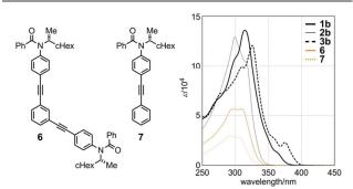
Figure 4. UV spectra of macrocycles  $\bf 1b$  (bold solid line),  $\bf 2b$  (thin solid line), and  $\bf 3b$  (bold dashed line), single-stranded substructure  $\bf 6$  (orange solid line), and diphenylacetylene  $\bf 7$  (orange dashed line), measured in CH<sub>2</sub>Cl<sub>2</sub> at room temperature.
