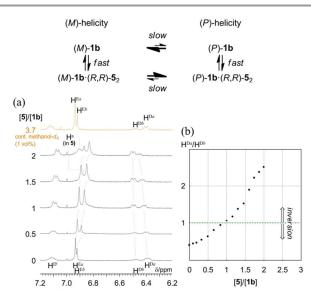
Figure 10. (a)  $^1$ H NMR spectra of (R,R,R,R)-**1b** (1 mM) in the presence of (R,R)-**5** (0-2 equiv., and 3.7 equiv. containing 1vol% methanol- $d_4$ ). All spectra were measured in CDCl $_3$  at 293 K. (b) Plot of the ratio of the populations of two species with (M)-por (P)-belicity versus equivalents of **5** added, based on phenylene protons H  $^{\rm DO}$  and H  $^{\rm C}$ .
