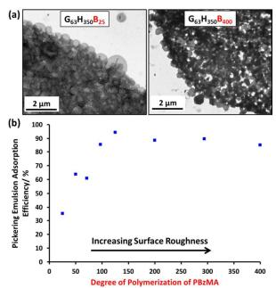
Fig. 5. (a) TEM images obtained for Pickering emulsions of n-hexane stabilized by aqueous vesicle dispersions of  $G_{63}H_{350}B_{25}$  and  $G_{63}H_{350}B_{400}$  triblock copolymer vesicles. (b) Plot of  $A_{\rm eff}$  vs. PBzMA DP in a series of  $G_{63}H_{350}B_z$  triblock copolymer vesicles (0.20 mM) with increasing surface roughness.
