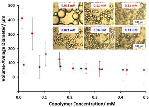
Fig. 4.Volume-average diameter (determined for n-dodecane droplets by laser diffraction) vs. copolymer concentration for ( $\blacklozenge$ ) linear  $G_{63}H_{350}$  diblock copolymer vesicles and ( $\blacklozenge$ ) framboidal  $G_{63}H_{350}B_{200}$  triblock copolymer vesicles. Inset shows representative optical microscopy images for selected emulsions prepared at the stated copolymer concentrations. The scale bars are valid for all six images.
