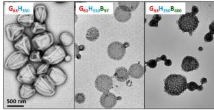
Fig. 1.Representative TEM images obtained for a series of framboidal  $G_{63}H_{350}B_z$  triblock copolymer vesicles (where z = 25-400) and also the precursor  $G_{63}H_{350}$  diblock copolymer vesicles. A 200 nm scale bar applies for the first ten images, while a 500 nm scale bar applies for the last three images.
