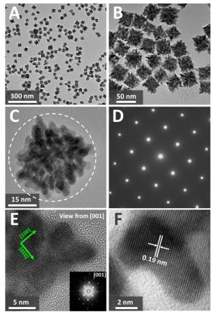
**Fig. 1** (A), (B) TEM images of dendritic  $Pt_3Cu$  cubes. (C) HRTEM and (D) corresponding electron diffraction (ED) pattern of a typical single crystalline dendritic  $Pt_3Cu$  cube. (E) Enlarged HRTEM image and corresponding FFT pattern of a corner of the single crystalline dendritic  $Pt_3Cu$  cube. (F) Further Enlarged HRTEM of a branch of the dendritic  $Pt_3Cu$  cube.
