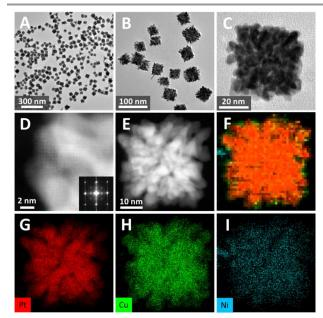
Fig. 5 (A), (B), (C) TEM images of dendritic PtCuNi cubes. (D) STEM and corresponding FFT pattern of a corner of single crystalline dendritic PtCuNi cube. (E) HAADF-STEM image and (F)-(I) EDX-Mapping of a single crystalline dendritic PtCuNi cube.
