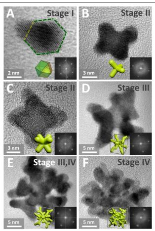
Fig. 3 (A)-(F) HRTEM images (insets show corresponding FFT patterns and cartoon models) of dendritic  $Pt_3Cu$  intermediates formed at different reaction stage.
