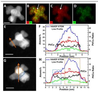
**Fig. 4.** (A) HAADF-STEM image and (B)-(D) quantified display of EDX-Mapping of an octapod intermediate. (E), (G) HAADF-STEM image and line scanning across a branch or branch connecting sites. (F), (H) HAADF-STEM line profiles (blue dots), elemental distribution of Pt (red lines) and Cu (green line) and Pt/Cu ratios (black lines) along the line scanning region marked in (E) and (G). Scale bars are 5nm.
