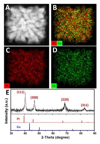
**Fig. 2** (A) HAADF-STEM image and (B)-(D) EDX-Mapping of a single crystalline dendritic  $Pt_3Cu$  cube. (E) XRD pattern of the single crystalline dendritic  $Pt_3Cu$  cubes. The standard diffraction peaks for Pt (JCPDS 03-065-2868) and Cu (JCPDS 03-065-9743) metals are also shown for comparison.
