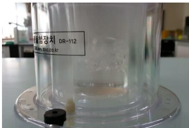
Figure 3. The phenomenon of water boiling in an evacuated container
