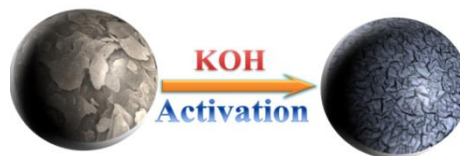
Fig. 1 Schematic diagram for the synthesis of ACs from coal
