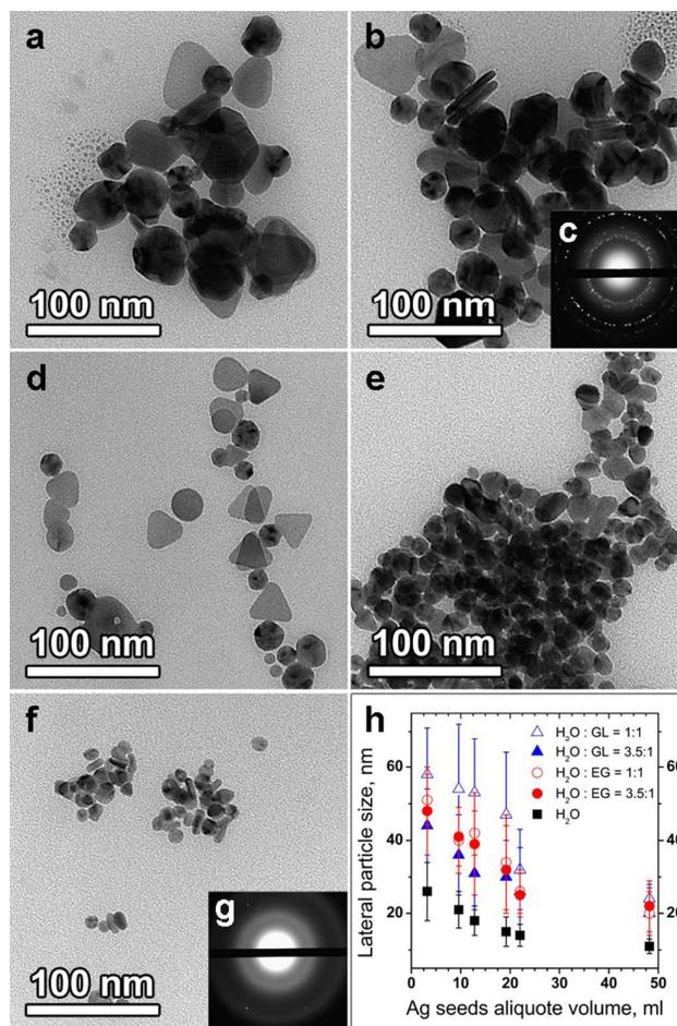
Fig. 1. TEM data of silver hydrosols synthesized with different aliquots of seeds of (a) 3.2 ml; (b) 12.8 ml, SAED is given in the (c) inset; (d) 25.6 ml, (e) 51.2 ml, (f) 76.8 ml, SAED is given in (g). (h) graphical representation of the particle size changes with Ag seeds aliquote volume in aqueous,  $\text{H}_2\text{O}$ -EG and  $\text{H}_2\text{O}$ -GL media.
