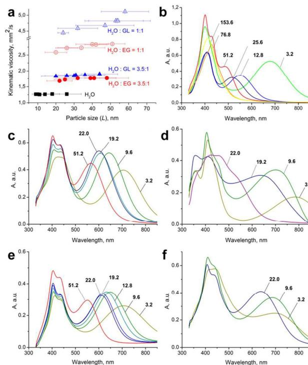
Fig. 2. Characteristics of silver inks. (a) Kinematic viscosity against a mean particle size (TEM data). UV-vis spectra of silver hydrosols and inks prepared in different liquors: (b) H<sub>2</sub>O, (c) H<sub>2</sub>O : EG = 3.5:1, (d) H<sub>2</sub>O : EG = 1:1, (e) H<sub>2</sub>O : GL = 3.5: 1, (f) H<sub>2</sub>O : GL = 1:1. The volumes of Ag seed aliquots (in ml) used in the sample syntheses are the labelling.
