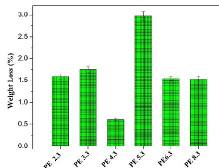
**Figure 10:** The bio-degradation of polyethylene. Dry weight loss of polyethylene after 90 days or 3 months
