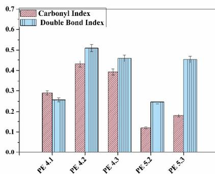
**Figure 5:** Carbonyl Index and Double Bond Index of control polyethylene and PE 4.1-PE 5.3
