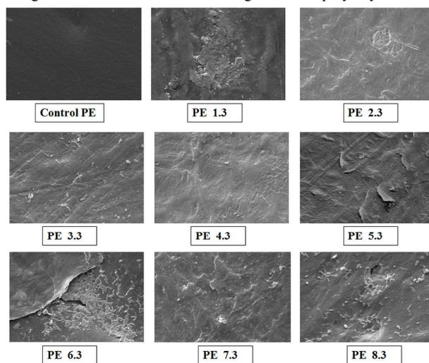
**Figure 9:** Scanning Electron Microscope image of PE 1.3-PE 8.3 and control polyethylene
