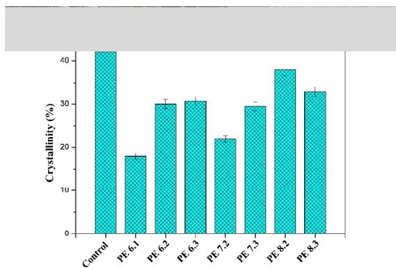
**Figure 8:** Crystallinity graph of control polyethylene and PE 6.1 to PE 8.3
