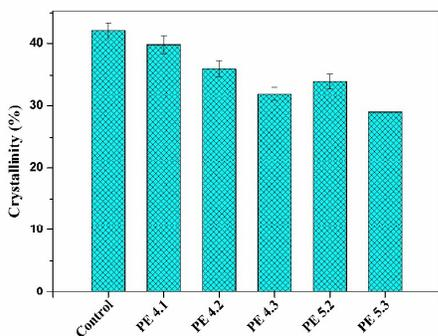
**Figure 6:** Crystallinity graph of control polyethylene and PE 4.1 to PE 5.3
