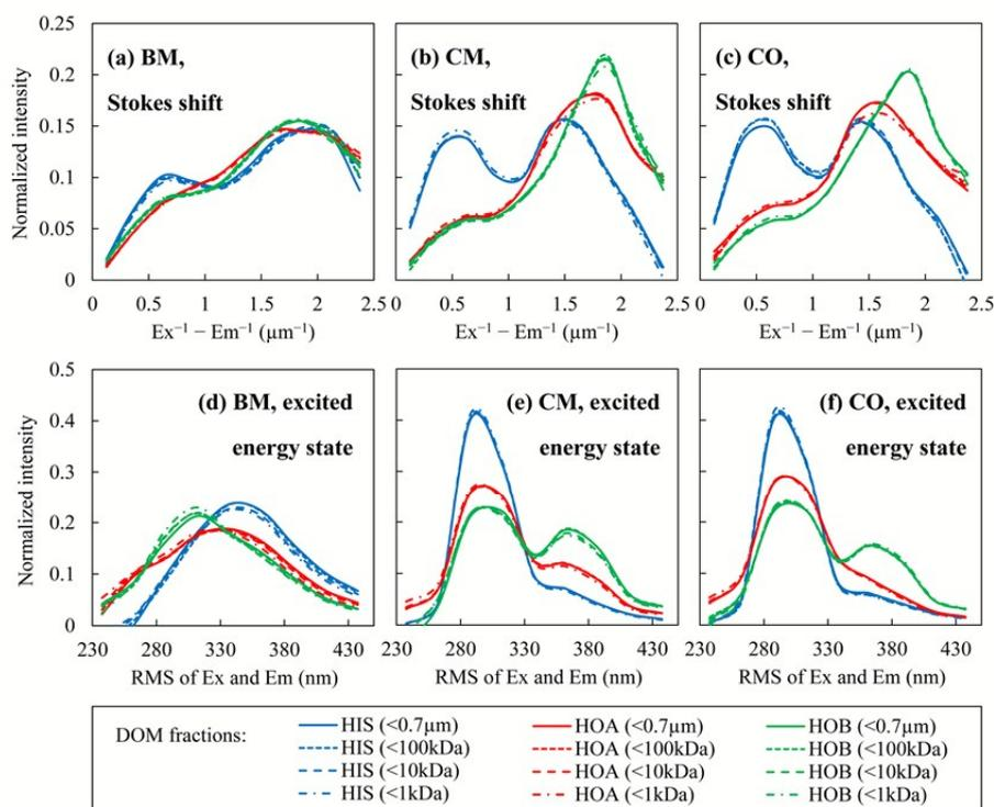
Fig. 5 Distributions of Stokes shift (measured by  $Ex^{-1}-Em^{-1}$ , a–c) and excited energy state (measured by RMS of Ex and Em, d–f) based on fluorescence intensity of DOM fractions.
