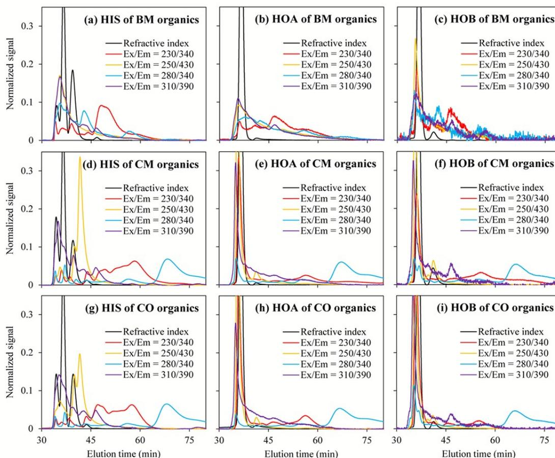
Fig. 6 HPSEC-FLD chromatograms of DOM fractions with different hydrophobicity from the BM, CM, and CO plants.
