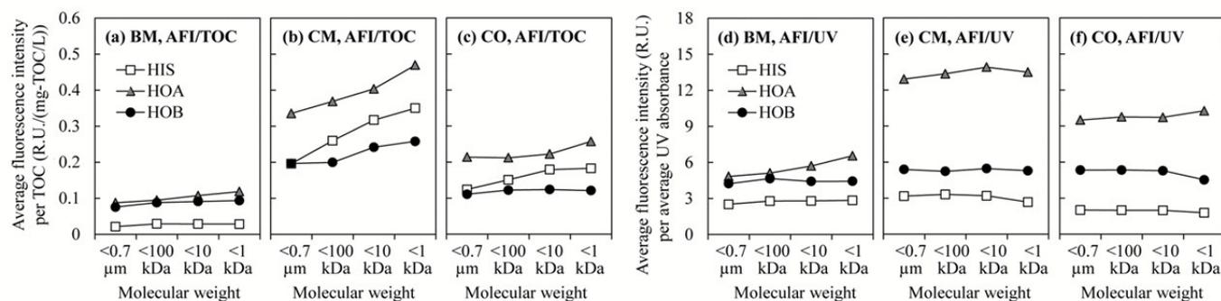
Fig. 4 Average fluorescence intensity per unit TOC (AFI/TOC, a–c) and average fluorescence intensity per average UV absorbance (AFI/UV, d–f) of DOM fractions from the BM, CM, and CO plants. The fluorescence intensity is averaged over the wavelengths of  $Ex = 200\text{--}400$  nm and  $Em = 250\text{--}500$  nm. The UV absorbance is averaged over the wavelengths of  $200\text{--}400$  nm.
