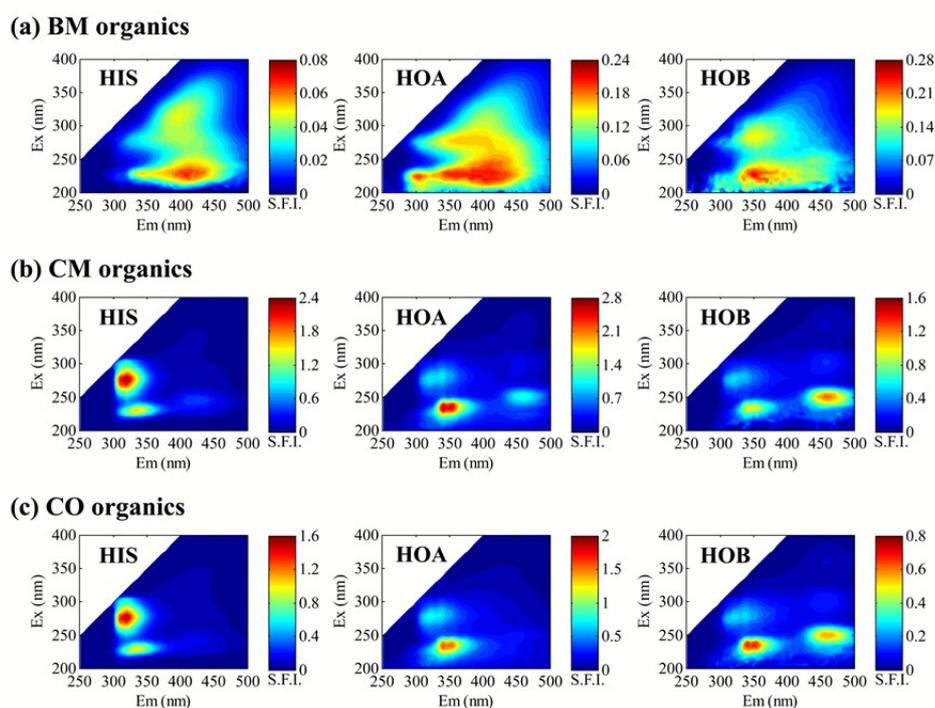
Fig. 3 Three-dimensional EEM fluorescence spectra of DOM fractions from the BM, CM, and CO plants.
