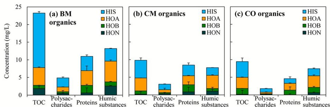
Fig. 1 Distribution of hydrophobic/hydrophilic fractions of DOM from the three wastewater treatment plants, denoted as (a) BM, (b) CM, and (c) CO plants. HIS = hydrophilic substances, HOA = hydrophobic acids, HOB = hydrophobic bases, HON = hydrophobic neutrals.
