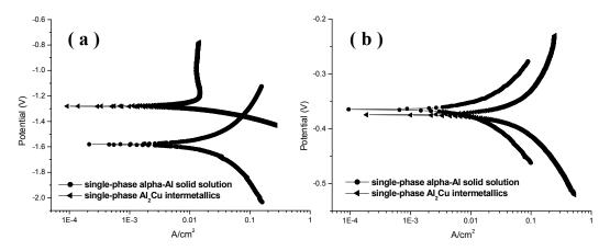
**Figure 6.** Tafel polarization curves of single-phase  $\alpha$ -Al solid solution and Al<sub>2</sub>Cu intermetallics (a) in the 10 wt.% NaOH solution, (b) in the 5 wt.% HCl solution.
