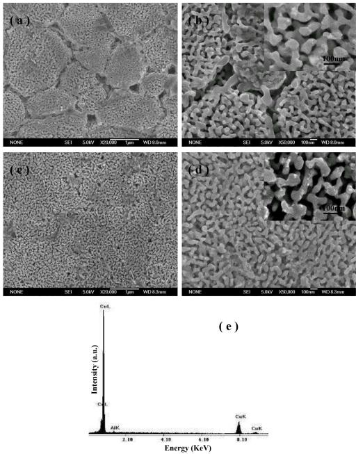
**Figure 2.** SEM images showing the microstructure of (a, b) quenching surface, and (c, d) free surface of NPCRs by dealloying of the Al 32 at.% Cu alloy in the 5 wt.% HCl solution at 75°C. Insets in parts b and d are their high-magnification images. (e) A typical EDX spectrum shows the composition of the resultant NPCRs.
