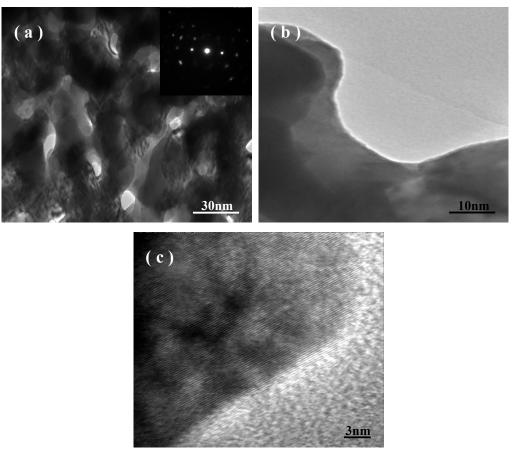
**Figure 5.** (a,b) TEM images show the porous structure in the channel walls of NPCRs by dealloying of melt-spun Al 32 at.% Cu alloy in the 10 wt.% NaOH solution at 15°C; (inset) SAED pattern corresponding to a ligament in part a; part b shows the smooth ligament surface morphology at a higher magnification. (c) HRTEM image shows lattice fringes extending throughout this ligament.
