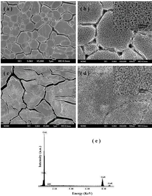
**Figure 4.** SEM images showing the microstructure of (a, b) quenching surface, and (c, d) free surface of NPCRs by dealloying of the Al 32 at.% Cu alloy in the 10 wt.% NaOH solution at 15°C. Insets in parts b and d are their high-magnification images. (e) A typical EDX spectrum shows the composition of the resultant NPCRs.
