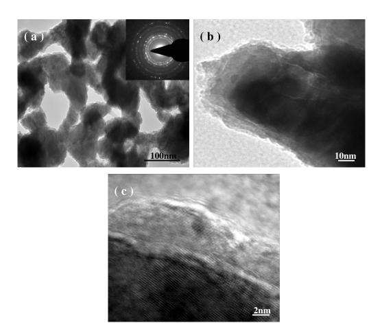
**Figure 3.** (a,b) TEM images show the porous structure in the channel walls of NPCRs by dealloying of melt-spun Al 32 at.% Cu alloy in the 5 wt.% HCl solution at 75°C; (inset) SAED pattern corresponding to a ligament in part a; part b shows the coarse ligament surface morphology at a higher magnification. (c) HRTEM image shows the crossed lattice fringes in the ligament.
