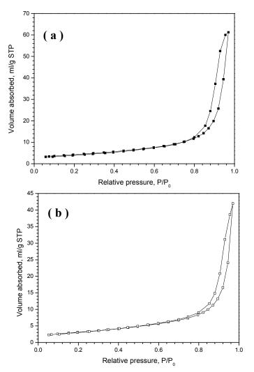
**Figure 7.** N<sub>2</sub> isotherms at 77 K for the NPCRs by dealloying of melt-spun Al 32 at.% Cu alloy (a) in the 10 wt.% NaOH solution and (b) in the 5 wt.% HCl solution.
