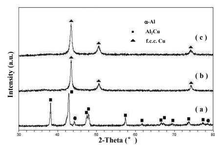
**Figure 1.** XRD patterns of melt-spun Al 32 at.% Cu alloy ribbons (a) before and (b-c) upon dealloying in the 5 wt.% HCl at 75°C and 10 wt.% NaOH solution at 15°C, respectively.
