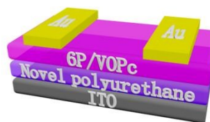
Fig. 1 Schematic of a bottom-gate top-contact para-sexiphenyl (p-6P) / vanadyl-phthalocyanine (VOPc) OTFTs device geometry.
