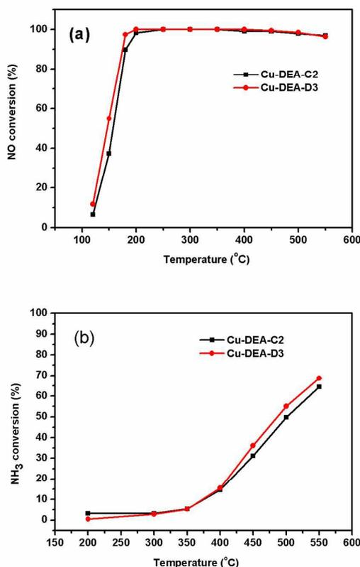
Fig. 6. (a) The standard SCR results with the feed gas of 500 ppm  $\text{NH}_3$ , 500 ppm  $\text{NO}$ , 5%  $\text{O}_2$ , and 5%  $\text{H}_2\text{O}$  with  $\text{N}_2$  as the balance. (b) The  $\text{NH}_3$  oxidation results with the feed gas of 500 ppm  $\text{NH}_3$ , 5%  $\text{O}_2$ , 5%  $\text{H}_2\text{O}$  with  $\text{N}_2$  as the balance. The volume hourly space velocity in all experiments was  $180,000 \text{ h}^{-1}$ .
