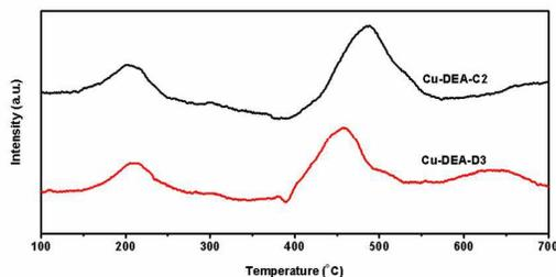
Fig. 5.  $\text{H}_2$ -TPR results of Cu-DEA-D3 and Cu-DEA-C2.
