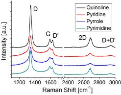
Figure 3. Raman spectra of N-doped graphenes synthesized at 500  $^{\circ}$ C.
