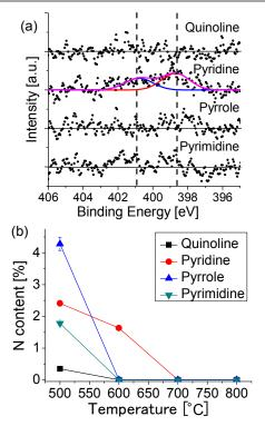
**Figure 5.** (a) XPS N 1s spectra of the graphenes synthesized at 600 °C. (b) Nitrogen content as a function of growth temperature for each of the source molecules.
