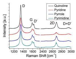
Figure 6. Raman spectra of the graphenes synthesized at  $600 \,^{\circ}\text{C}$ .
