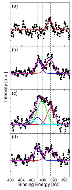
**Figure 4.** XPS N 1s spectra of N-doped graphenes synthesized at 500 °C from (a) quinoline, (b) pyridine, (c) pyrrole, and (d) pyrimidine. Each spectrum is fitted with three Gaussian functions: pyridinic- (red line), pyrrolic- (green line), and graphitic-N (blue line).
