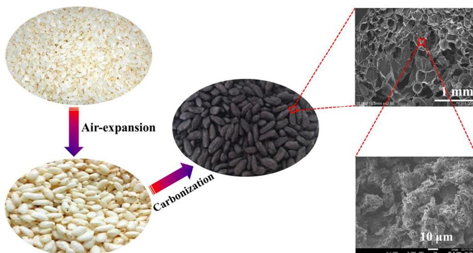
**Fig. 1 - Schematic illustration of the air-expansion method for hierarchically porous carbon aerogel from rice.**
