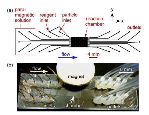
**Fig. 2** (a) CAD design of the microfluidic device, featuring a reaction chamber fed by 10 inlet channels, including a flow focussing section for the introduction of reagents and functionalised polymer particles, and with 9 outlet channels. (b) Photograph of the glass device with interfaced tubing and a 20 mm  $\emptyset$  x 5 mm NdFeB magnet placed on the chip, next to the chamber.
