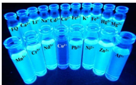
Figure 2 Fluorescence responses of FQ1 in the presence of different metal ion in DMSO: MeOH (v/v, 1:9) solution.
