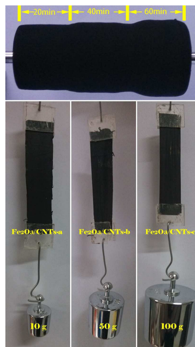
Figure 11. Strength test of \text{Fe}_2\text{O}_3/\text{CNTs} -a, b and c.
