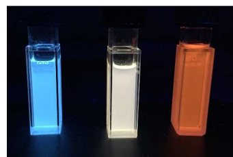
Figure 4: Changes in the colour of a \text{CH}_2\text{Cl}_2 solution of 1 ( c = 2.2 \cdot 10^{-4} M, left) after the addition of 50 equivalents (middle) and 1000 equivalents of TFA (right). Photographs were taken in the dark upon irradiation with a hand-held UV lamp ( \lambda_{\text{em}} = 366 nm).
