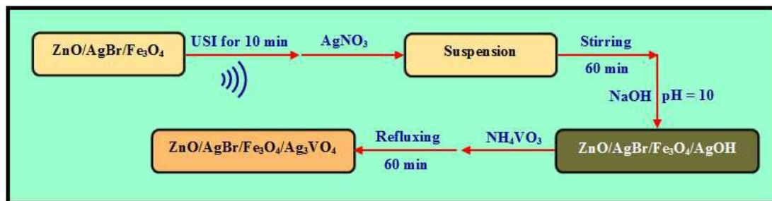
Scheme 1. The schematic diagram for preparation of the ZnO/AgBr/Fe 3 O 4 /Ag 3 VO 4 nanocomposites.
