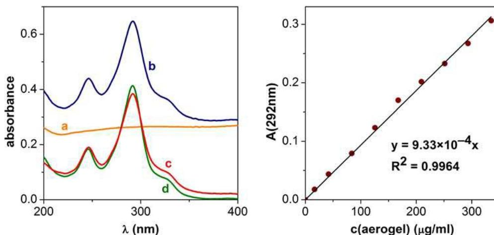
**Figure 6.** A: a) The spectrum of a well stirred aerogel suspension (331 μg/mL), b) the spectrum recorded immediately after the addition of MB to this suspension, c) the difference spectrum of these two, d) the spectrum of the pure MB solution (10.2 μM). B: Absorbance versus concentration plot of the aerogel suspension. The absorbance is due to the light scattering of the suspension.  $c(\text{NaH}_2\text{PO}_4 + \text{Na}_2\text{HPO}_4) = 50$  mM; pH = 6.91; 25 °C; 1000 rpm stirring.
