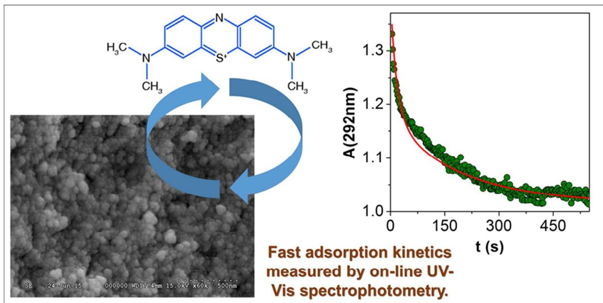
**Pore network and adsorption properties of mesoporous silica aerogel: a mechanistic study on the timescale of seconds.**
