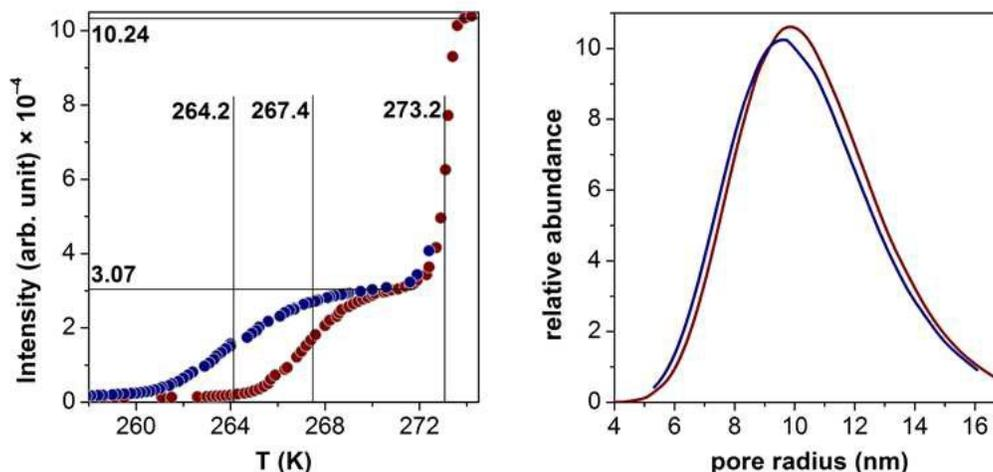
**Figure 3.** Melting (red) and freezing (blue) curves of the aerogel suspension measured by NMR cryoporometry. The position of the inflection points and the height of the plateaus are indicated in the plot. B: Log-normal size distribution of the pores in the aerogel particles. Reconstructed from Fig 3A assuming spherical pores (red: from the melting curve, blue: from the freezing curve).
