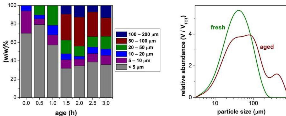
**Figure 2.** Aging of the aerogel suspension. A) The size distribution of aerogel particles ( $< 10 \mu\text{m}$ ) and aggregated blocks ( $> 10 \mu\text{m}$ ) measured by conventional microscopy. Each colored column represents the weight percent contribution of a given fraction. B) Size distribution by the volume of aerogel particles in a fresh and in an aged suspension measured by dynamic light scattering (DLS).
