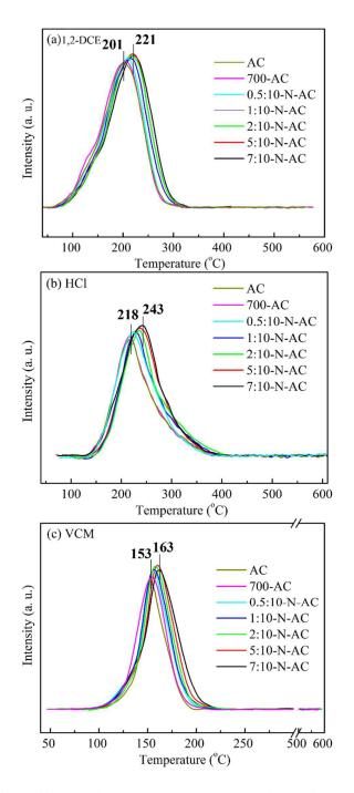
Fig. 2. TPD profiles of the catalysts. (a) 1,2-DCE-TPD, (b) HCl-TPD, (c) VCM-TPD
