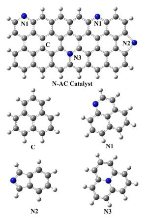
2 Fig. 3. The structures of various N species in the N-doped AC catalysts. C: graphene
