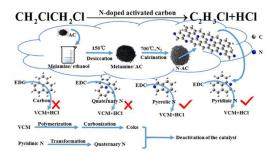
Pyridinic and pyrrolic nitrogen dopants in the N-AC catalyst can adsorb EDC and increase the activity for EDC dehydrochlorination.
