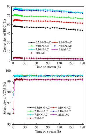
4 Fig. 1. 1,2-DCE conversion and the selectivity to VCM over different catalysts.
