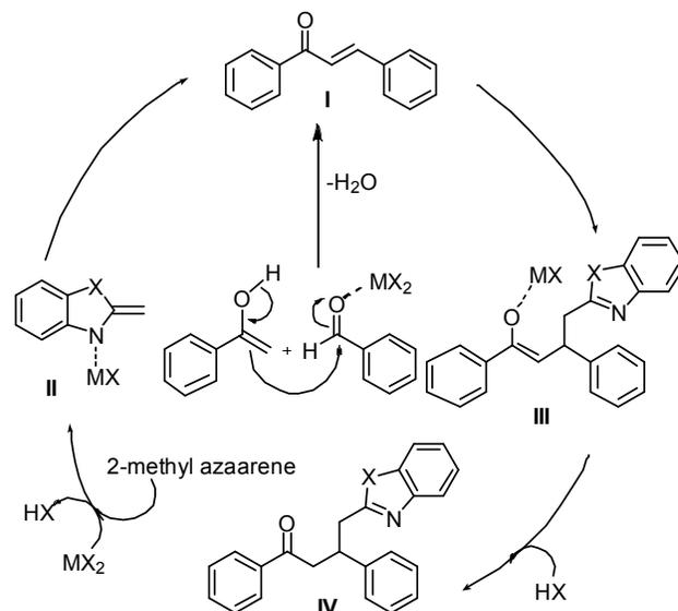
**Scheme 4** Plausible mechanisms for the synthesis of  $\beta$ -azaarenes substituted ketones.
