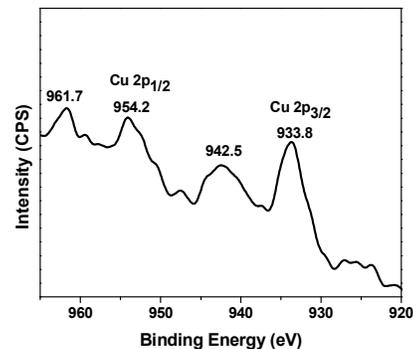
Figure 8: High resolution XPS of Cu 2p region in Cu@Fe<sub>2</sub>O<sub>3</sub> MNPs
