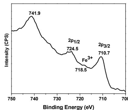
Figure 9: High resolution XPS of Fe 2p region in Cu@Fe<sub>2</sub>O<sub>3</sub> MNPs
