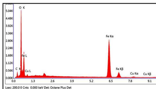
**Figure 5:** EDAX elemental analysis of Cu@Fe<sub>2</sub>O<sub>3</sub> MNPs
