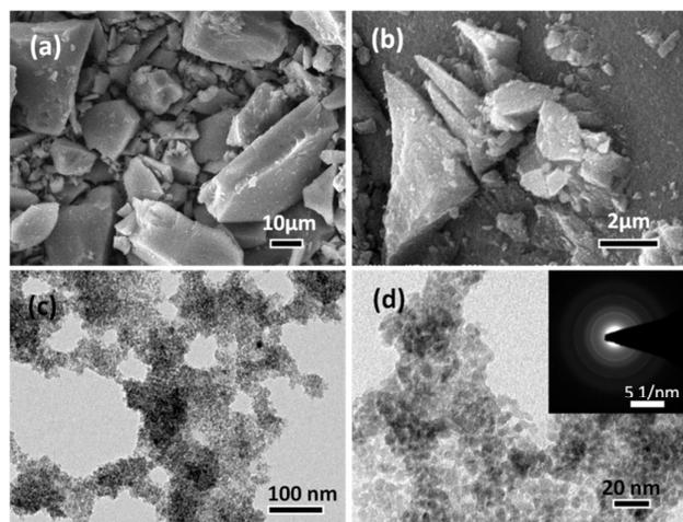
Figure 6: SEM (a, b) and TEM (c, d) images of Cu@Fe<sub>2</sub>O<sub>3</sub> MNPs
