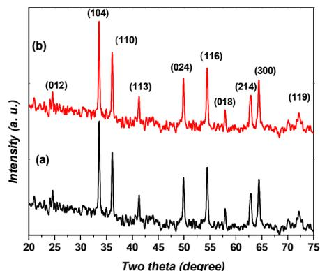
**Figure 3:** XRD of (a) fresh and (b) recycled Cu@Fe<sub>2</sub>O<sub>3</sub> MNPs
