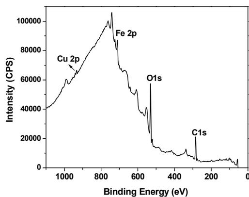
Figure 7: Survey X-ray photoelectron spectra of Cu@Fe<sub>2</sub>O<sub>3</sub> MNPs
