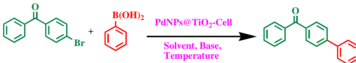
Scheme 1. Suzuki-Miyaura reaction catalyzed by PdNPs@TiO 2 -Cell
