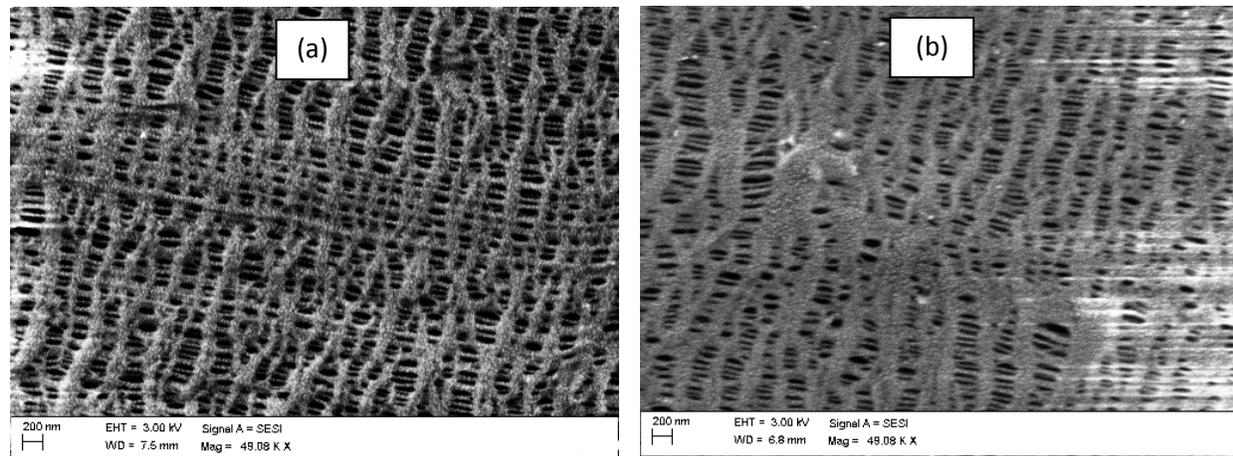
**Figure 3:** FESEM images of (a) control PP film and (b) Poly(EPMA)-g-PP film
